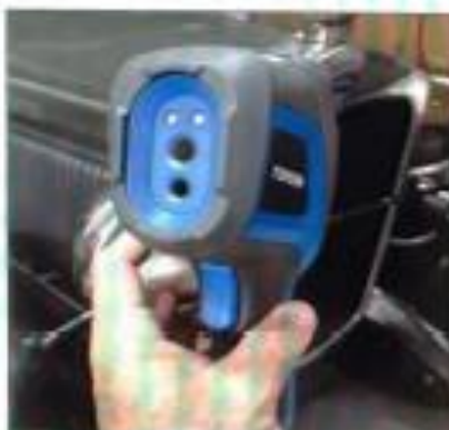
Photo 2. Sensors in the front detect heat from various sources.
